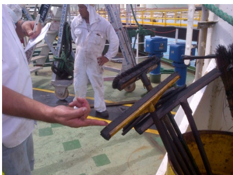
Picture 9 – SOPEP Equipment Manifold Soaked with Oil
