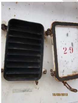
Picture 2 – Broken Damper
