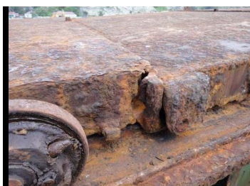
Picture 2 – Broken Damper
