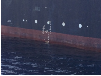
Pictures 4 – Load Line Marks Not Properly Marked
