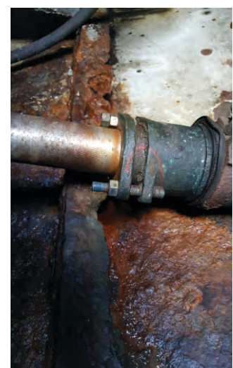
leaking stern gland and wasted shell angle framing below
