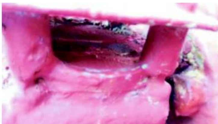
Flame Arrestor Screen Partially Painted
