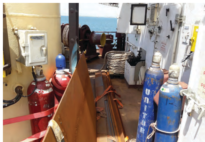
Improper storage of acetylene and oxygen bottles (spontaneous combustion when both gasses combine)
