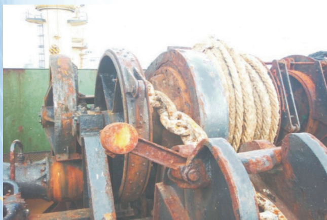
WINDLASS AND GYPSY HEAVILY CORRODED
