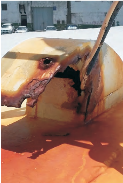
Corroded vent casing
