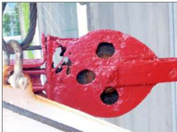
Life Boat Pulley Corroded
