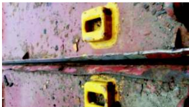
Cargo Hatch Cover Joint Gasket Damage
