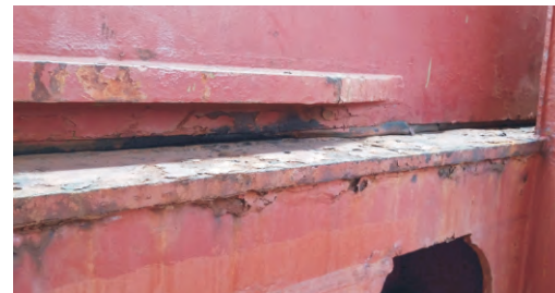
Hatch cover flexible rubber seal damaged
