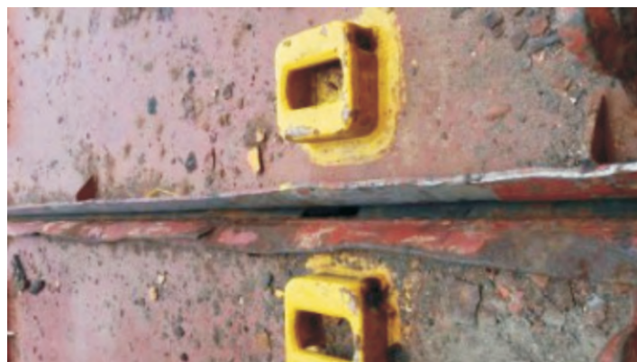
Cargo Hatch Cover Joint Gasket Damage
