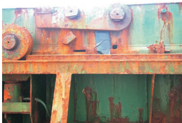
SEALING TAPE USED AND HATCH DOG NOT IN PROPER POSITION
