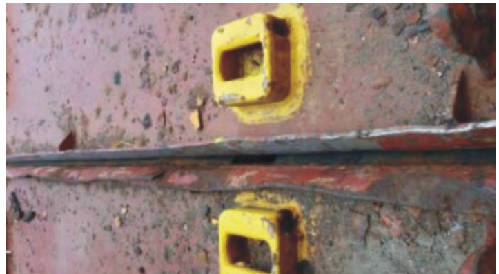
Cargo Hatch Cover Joint Gasket Damage
