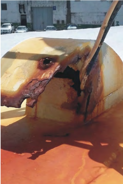
Corroded vent casing
