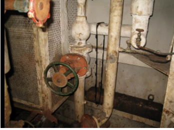
Picture 1 - Bilge discharge directly to the sea
