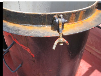
Picture 3 - Cargo Tank lid securing devices broken
